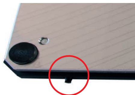
Workpiece carrier with shock absorber
