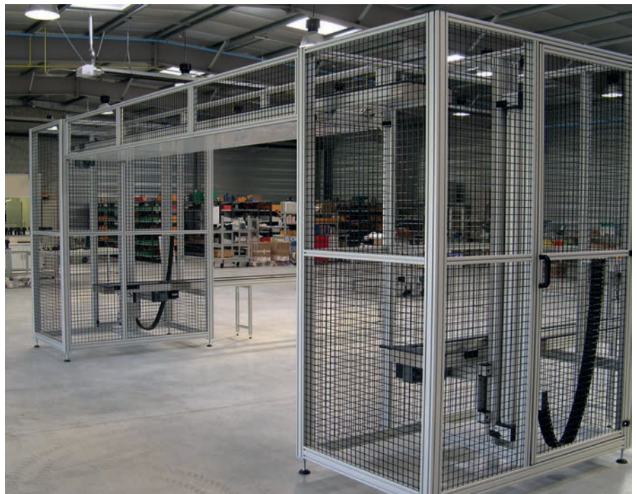
Bridge built from two transfer systems
