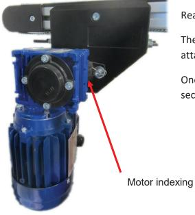
Reassemble the motor in the desired position.
