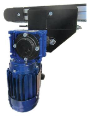
The motor is located next to the belt at the required place.
