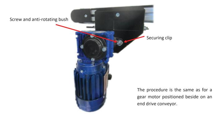
Case of a gear motor positioned below for an end drive conveyor
