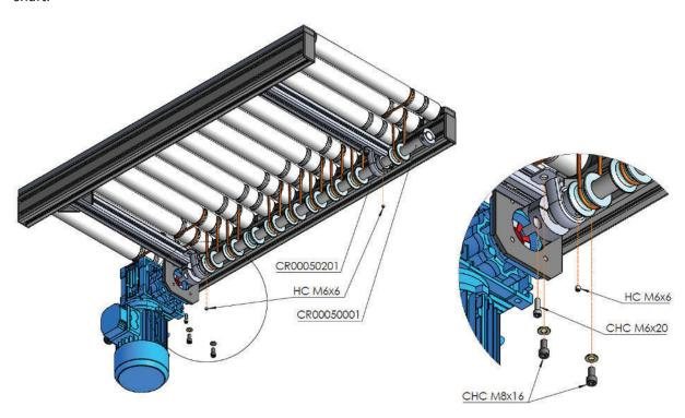
The driving shaft can now be removed up to the roller  $\emptyset$ 30 involved by the round belt replacement.
