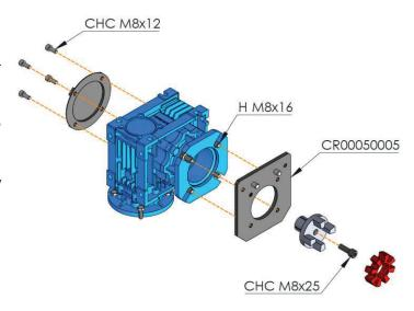
Before reassembling, degrease the hollow shaft of the new gearbox and the half elastic jaw coupling.
