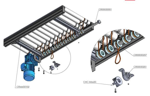
On top of the conveyor, screw off the screws FHC M5x12 to release the 2 aluminum angles CR00050103, then remove the rollers in contact with the round belt who need to be replaced.
