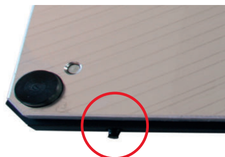
Workpiece carrier with shock absorber
