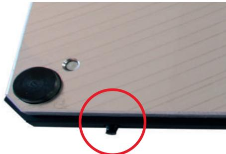
Workpiece carrier with shock absorber
