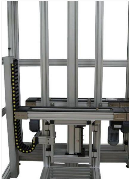
Lift for two transfer system units
